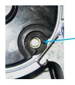
Primer Cup fits Hole in Platform without dragging and is concentric with the "U" shaped Shellplate opening/slot
