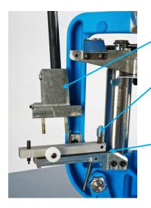
Remove all together--Primer Mag Shield, Cap, and Early Warning Alarm Assembly.
