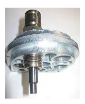
• Loosen the Shellplate Bolt locking Set Screw in the left side of the Main Shaft. Remove Ejector Spring. Remove the Shellplate Bolt and Shellplate.
