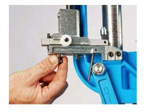
Replace the Operating Rod and re-attach Slide Return Spring.
