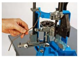
Perform a single primer feed test as previously described to verify correct operation of the Primer Feed Assembly.
