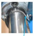
Carefully remove Indexer Return Spring from the two pins
