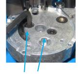
Remove Platform Mounting Screws and the Platform
