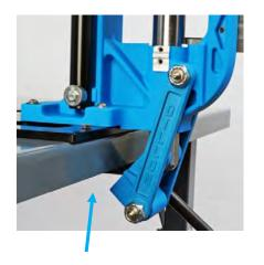
Note ¾" clearance required for the Crank and Operating Handle if mounting XL750 base directly to the bench
