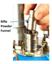
5.8.3 Place the Powder Measure onto the Powder Die and lightly tighten the two clamp screws.
