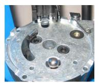
Reinstall Index Pawl and Spring and Index Ball and Spring
