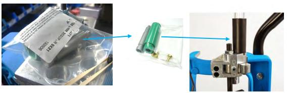
Note: Casefeed Adapter are different colors for different calibers
