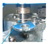
Tighten both Platform Mounting screws while keeping the Alignment Fixture pin engaged in the Primer Hole
