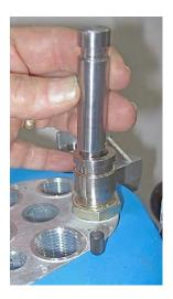
Lower the Platform as little as possible, keeping the Alignment Pin engaged while tightening the two Platform Mounting Screws. Lower the Platform down and tighten both Mounting screws snugly—8-10 ft-lbs. while not allowing the Platform to shift while tightening.
