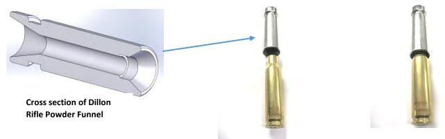
Rifle case neck fits up inside Caliber Specific Powder Funnel to Activate Powder Measure
