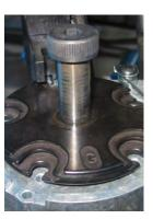
• Remove the Indexer Return Spring, Index Ball and Spring and the Index Pawl ("Tomahawk") and its Spring. Note the direction the Pawl faces. Remove the two Platform Mounting Screws
